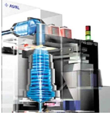
Figure 1: Semiconductor Wafer Stepper with an Upgradeable Projection Lens Module
